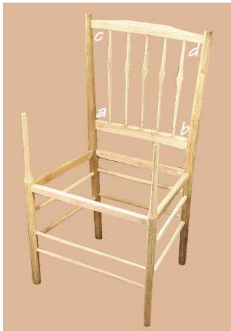
▲ Pic. 7 On the unfinished chair, spacing the back spindles raised an arithmetical problem
